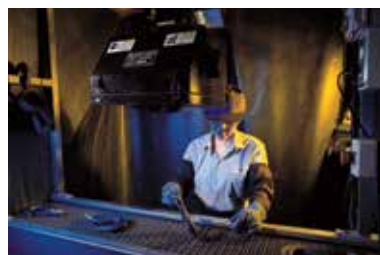
Magnaflux Crack Detection
